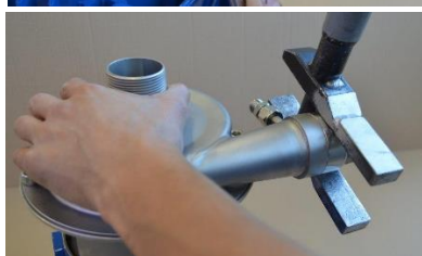
Fig. 3.5.8 Unscrew the connection adaptor [1364].
