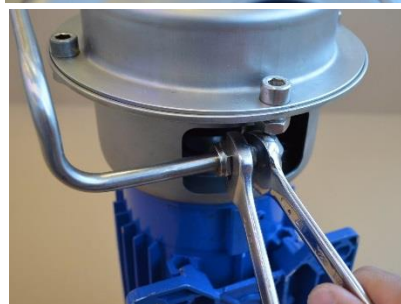
Fig. 3.5.5 Loosen the screw on the elbow union [1367].
