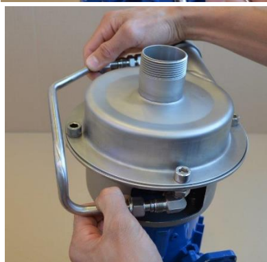
Fig. 3.5.6 Remove the metal pipe [1363].
