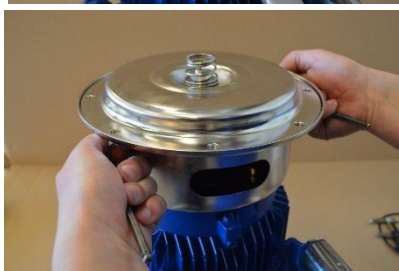
Fig 3.5.15 Carefully remove the back casing [126]. The static part [15B] of the mechanical seal will remain in the back casing.
