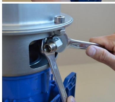
Fig. 3.5.7 Unscrew and remove the elbow union [1367].
