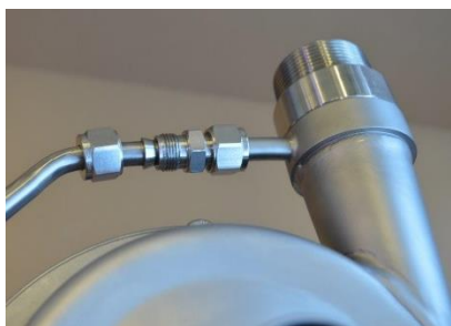
Fig. 3.5.4 Release the metal pipe [1363].
