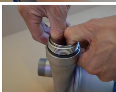
Fig. 3.5.9 Take out the strainer [1361] and the O-ring [1365].
